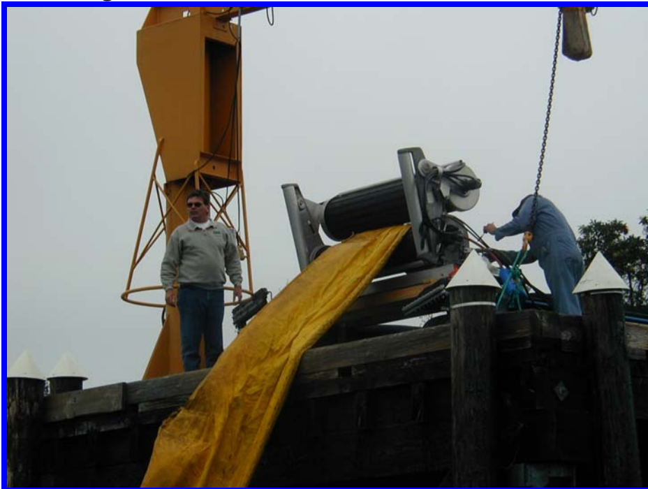
Pictured is 42" foam-filled oil containment boom being recovered at 100ft/min with a 26ft lift
