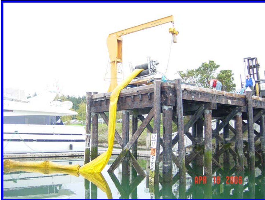
Pictured is 42" foam-filled oil containment boom being recovered at 100ft/min with a 26ft lift
